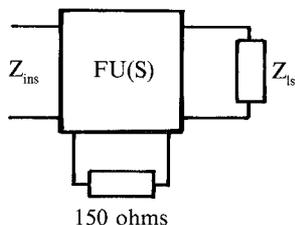
$Z_{ins}$ : Input impedance of the FU(S) at the voice channel interface.
