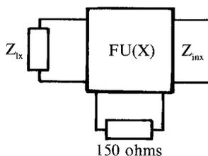
$Z_{inx}$ : Input impedance of the FU(X) at the voice channel input.
